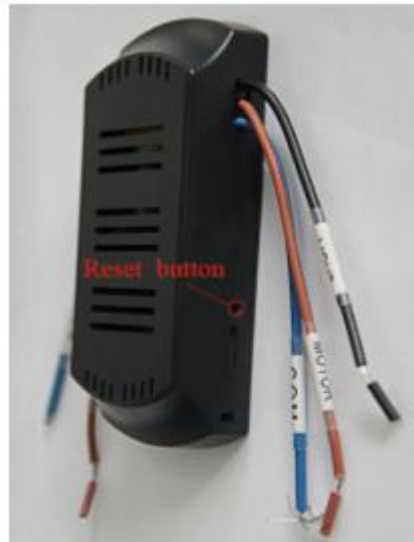
Fig. 4 Reset Button of uCF281 controller
