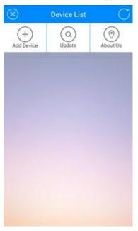
2.2 Click "Add Device" button, enter Device ID and Password. Every receiver has a unique ID assigned at factory, and the default Password is 1234567. The password can be changed by the user once the initial setup and operation are completed.
