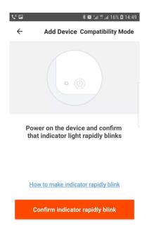
**Step 3:** If Internet configuration failed in Step 2, please select "Compatibility Mode (AP Mode)" to configure network. Long press the Reset button of the transmitter or the receiver, and switch it to slowly blink. If Internet configuration are successful in Step 2, skip Step 3.
