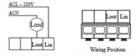
Fig. 3 BRT-413 Wiring Diagram
