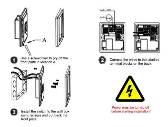
Fig. 4 BRT-413 Installation Guide
