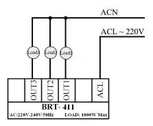
Fig. 4 Wiring Diagram of Wall Mount Unit
