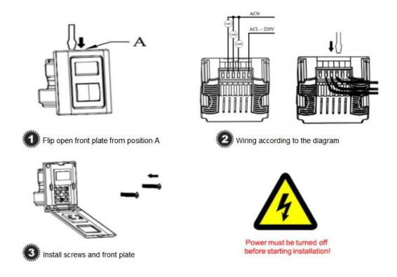
Fig. 5 Installation Guide of Wall Mount Unit
