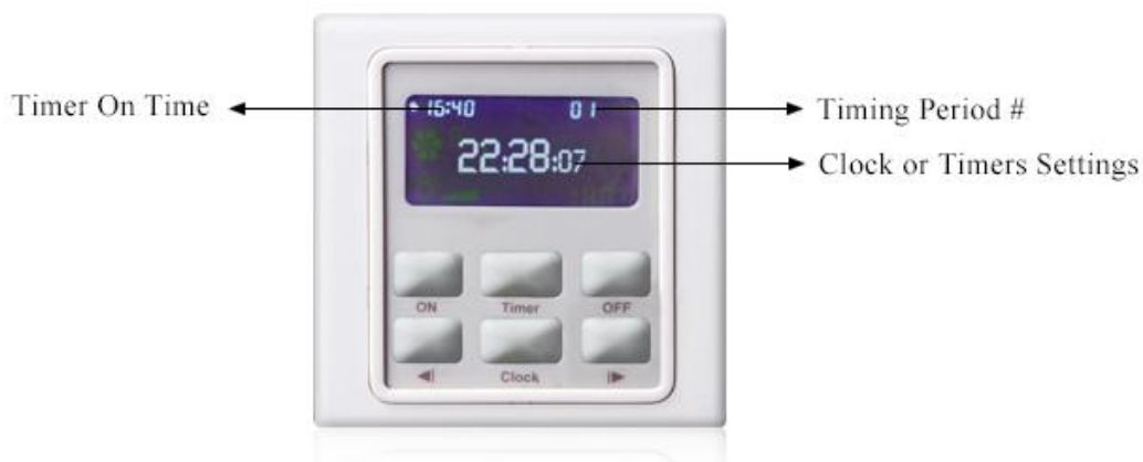
Fig.3 Front Control Panel and LCD Display
