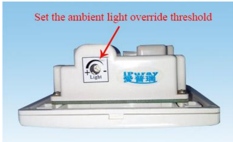
Fig. 5 Adjustment of Ambient Light Override Threshold
