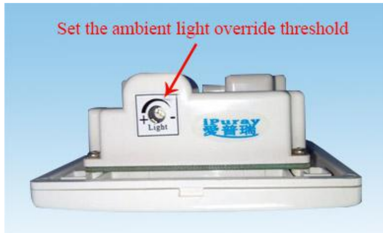
Fig. 5 Adjustment of Ambient Light Override Threshold
