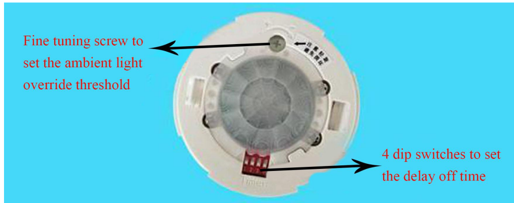
Fig. 6 Dip Switches and Fine Tuning Screw
