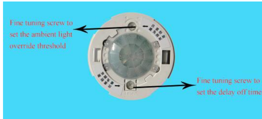
Fig. 6 Fine Tuning Screws for Initial Setups
