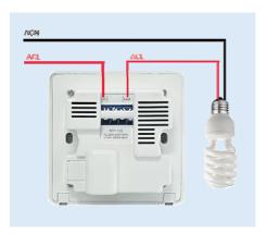
Fig. 4 BRT-120 Timer Switch Wiring Diagram
