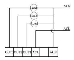
Fig. 4 BRT-107 Timer Switch Wiring Diagram
